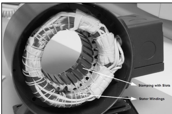
Fig. 2 Stator structure of a BLDC motor [10].
